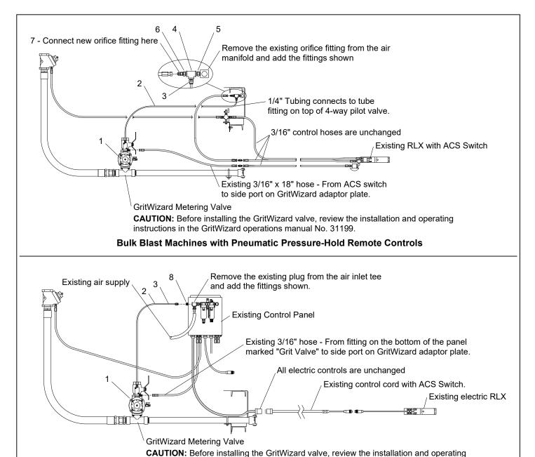
**Bulk Blast Machines with Electric Pressure-Hold Remote Controls**
