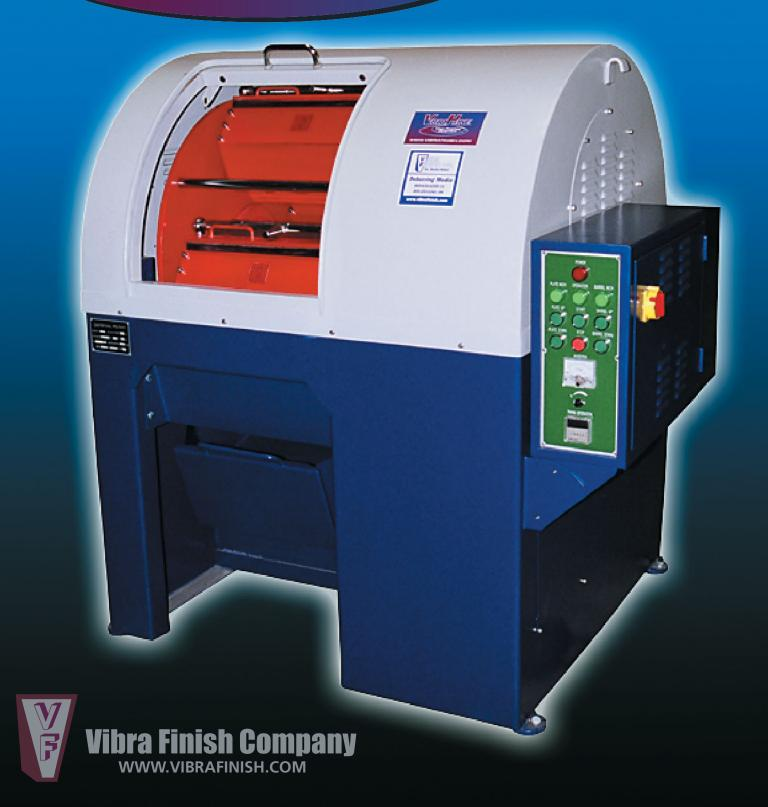
The CB-100 centrifugal barrel finisher features high efficiency, a wide speed range, ease of operation and low noise levels all in an attractive machine enclosure. Revolving barrel groups rotate in opposite directions on independent axis driven by the planetary drive system. Media and working parts are worked under dual centrifugal forces which create an efficient and uniform chamfer, debur or polishing action.
