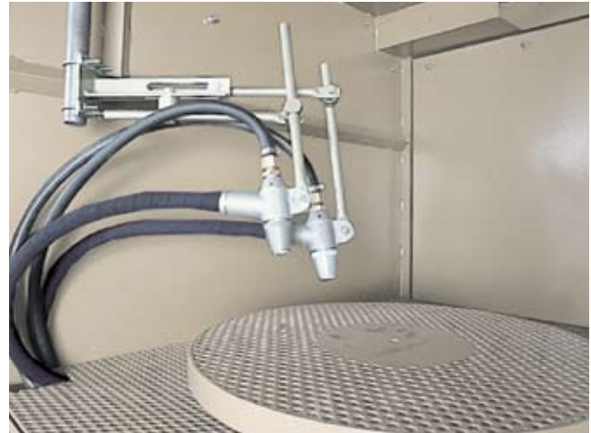
Fixed gun holder frees operator to manipulate parts.
