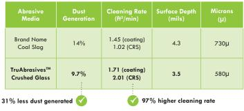
Results were verified by an independent testing laboratory on cold rolled steel.
