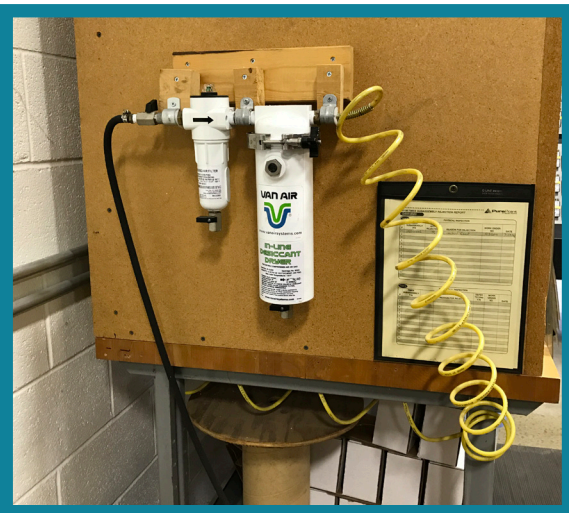
An Inline Desiccant Dryer and F200-15 filter being used on a ultrasonic welder.
