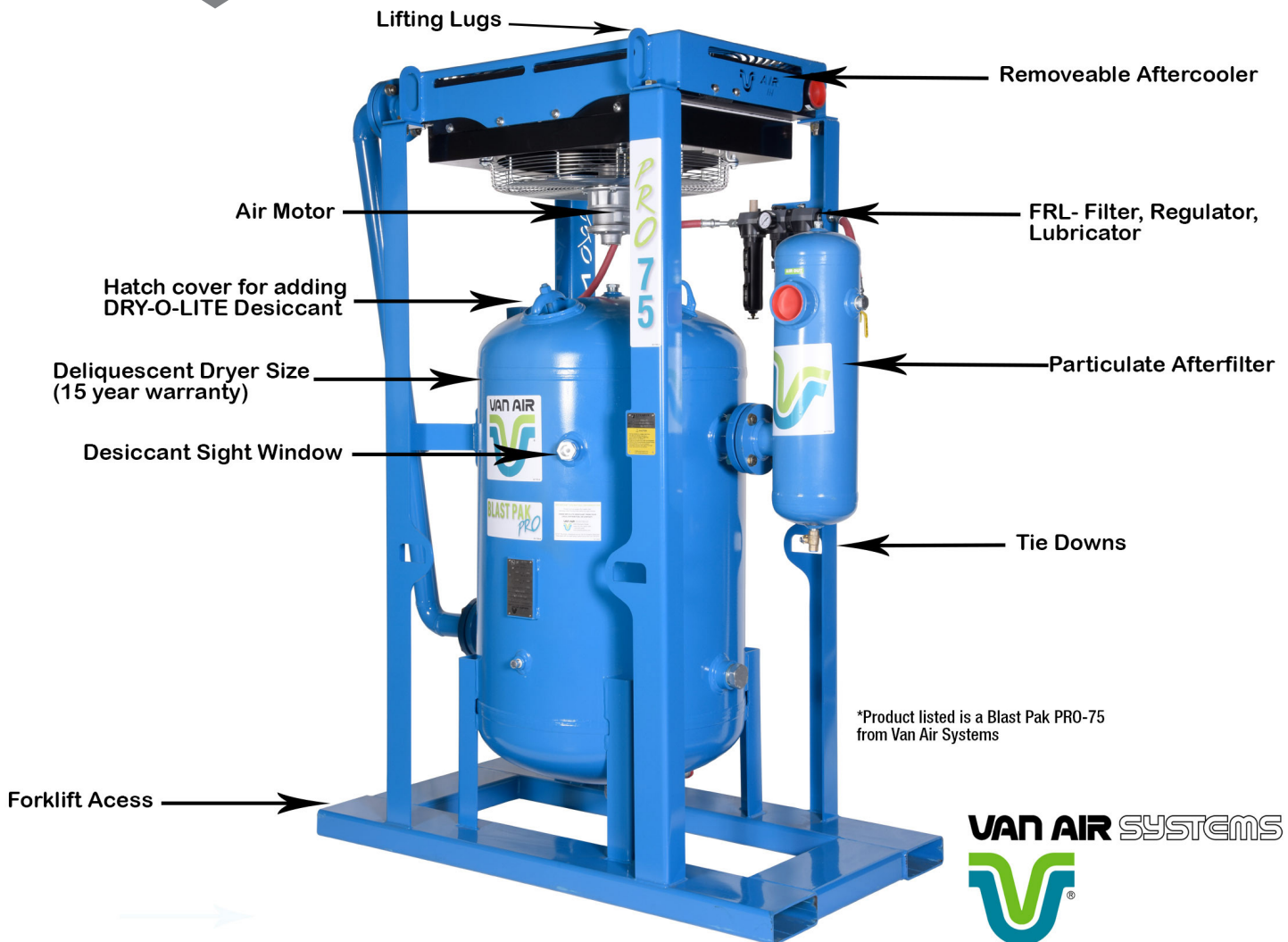
Portable Compressed Air Dryer Diagram
